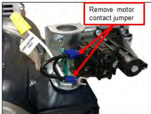
3. Remove motor contact jumper, leaving motor HOT in terminal. Retighten motor HOT wire in terminal.
