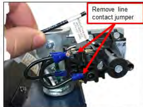
2. Remove line contact jumper and HOT wire placeholder.
