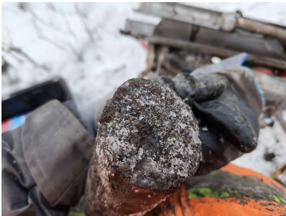
Photo A - 14. BH-03 Representative Sample of Vr Ice Classification encountered From Sample 6 @ 15-Feet
