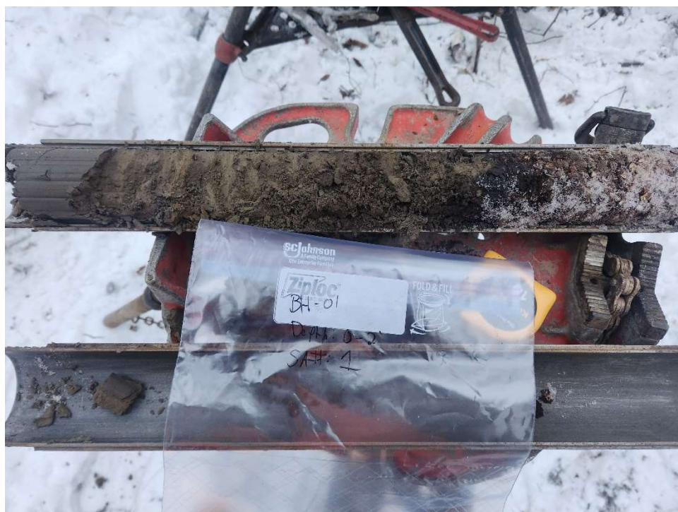
Photo A - 1. BH-01 Representative Sample of Surficial Organics and Silt (ML) from 0 to 6-Feet
