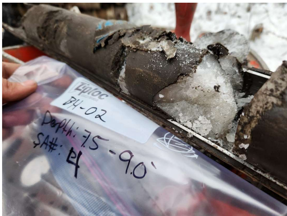
Photo A - 8. BH-02 Representative Sample of the ICE Mass encountered from 7 to 9-Feet and Similar Conditions at 51-Feet
