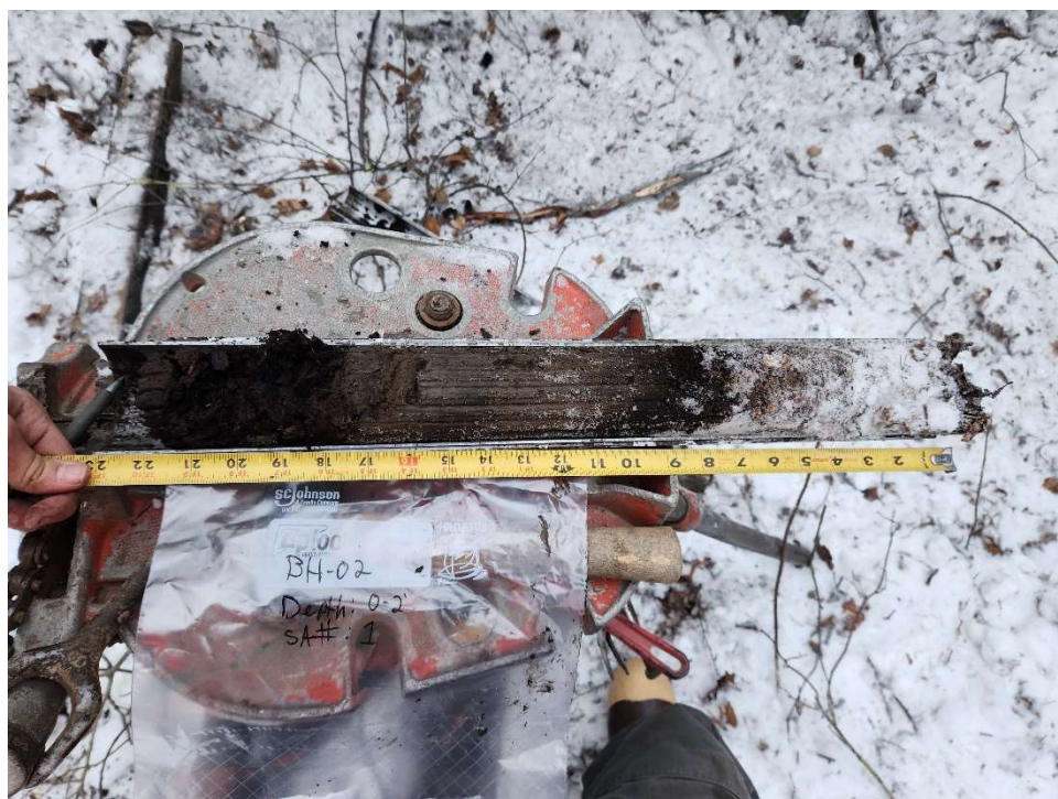
Photo A - 6. BH-02 Representative Sample of Surficial Organics and Silt (ML) from 0 to 3-Feet
