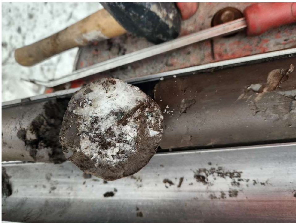
Photo A - 5. BH-01 Example of Vx Classification from Sample 11 at 40-Feet
