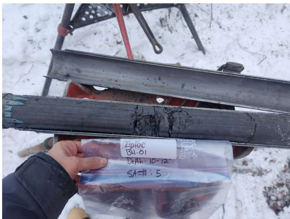
Photo A - 2. BH-01 Representative Sample of Frozen Silt (ML) from 6 to 51.1-Feet
