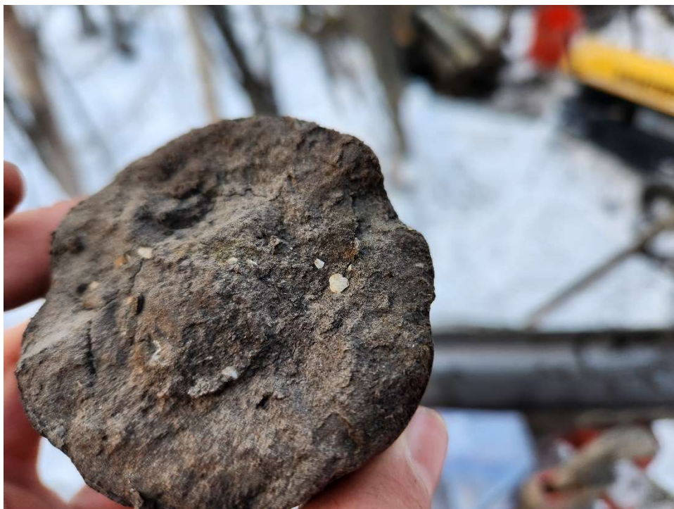
Photo A - 16. BH-03 Shells encountered at 40 – Feet
