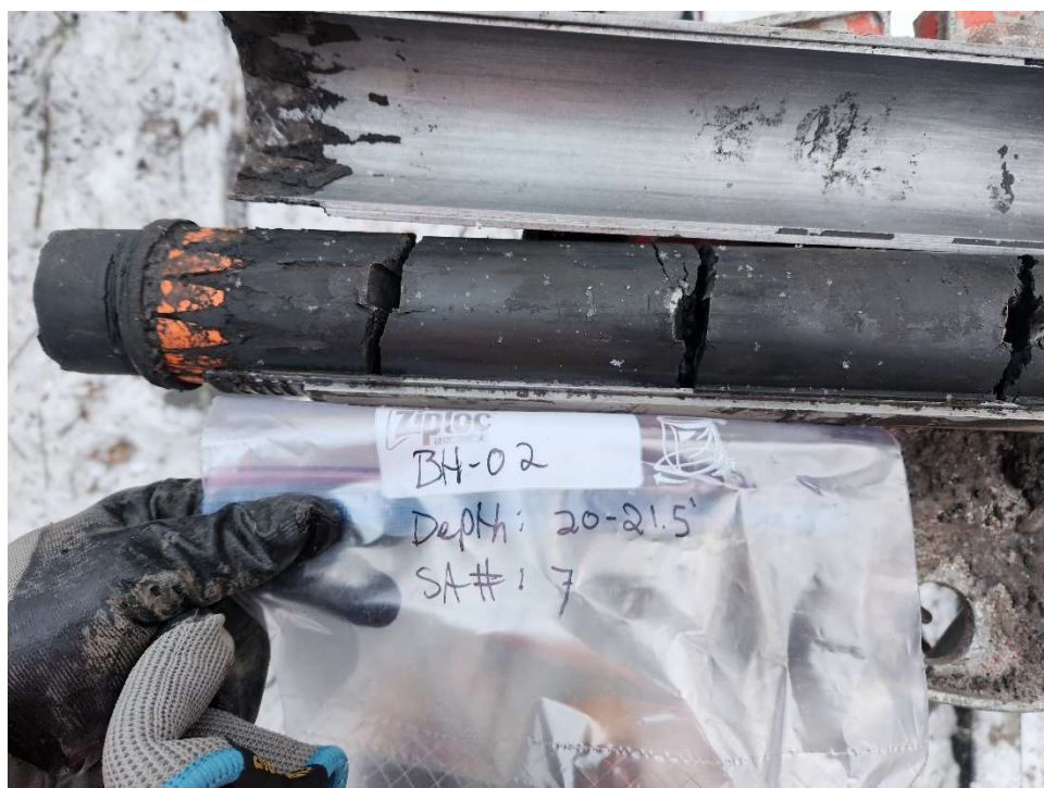
Photo A - 9. BH-02 Representative Sample of Frozen Silt (ML) from 9 to 51-Feet
