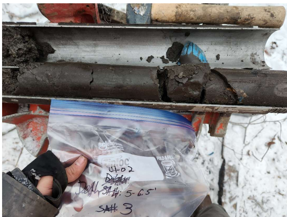
Photo A - 7. BH-02 Representative Sample of Frozen Silt (ML) from 6 to 7-Feet
