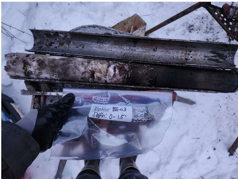
Photo A - 10. BH-03 Representative Sample of Surficial Organics and Silt (ML) from 0 to 3-Feet
