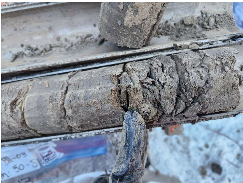
Photo A - 17. BH-03 Close up Very Dry Silt (ML) at 43 to 51.5-Feet. Possibly unfrozen.
