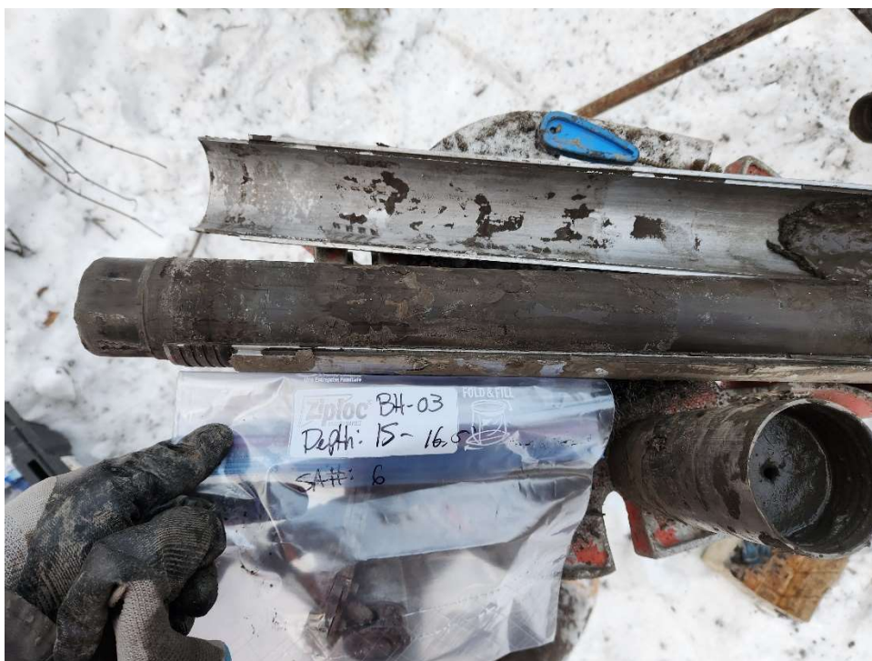
Photo A - 12. BH-03 Representative Sample of Frozen Silt (ML) from 9 to 43-Feet
