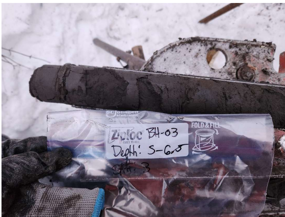
Photo A - 11. BH-03 Representative Sample of Silt (ML) from 0.5 to 9-Feet
