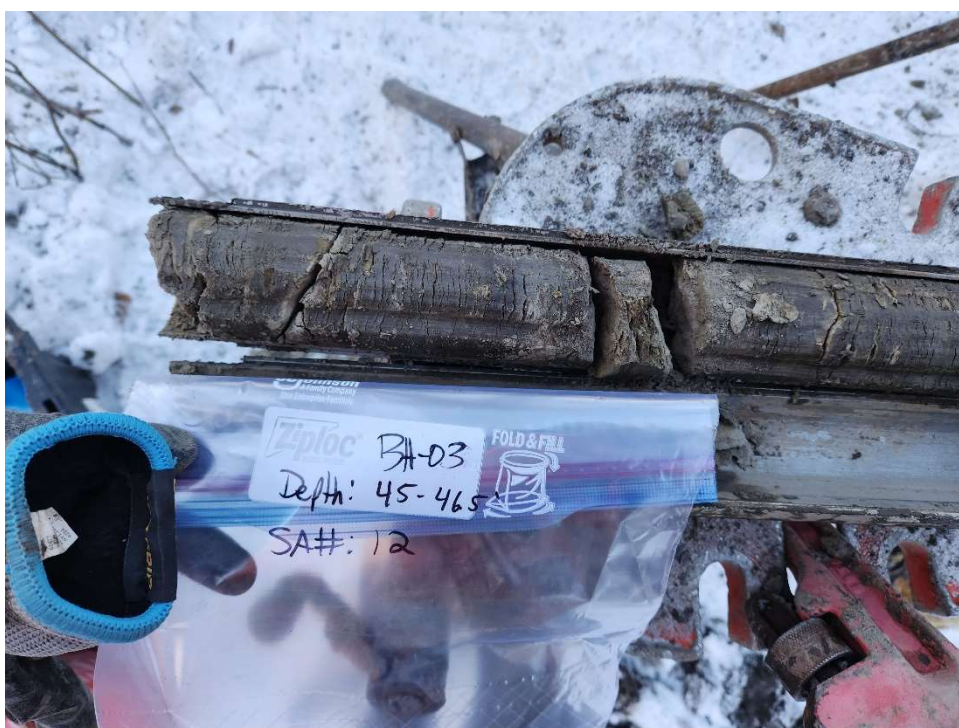
Photo A - 13. BH-03 Representative Sample of Very Dry Silt (ML) from 43 to 51.5-Feet. Material is possibly non-frozen
