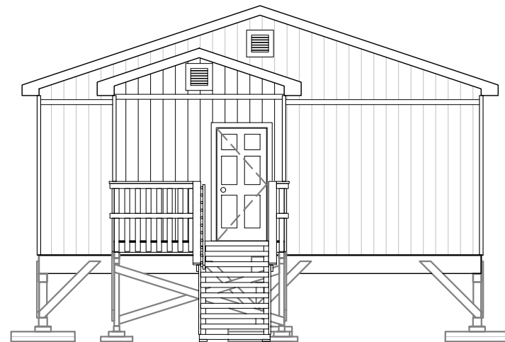
2 FRONT ELEVATION SCALE: 1/8"=1'-0" 11x17 SHEET
