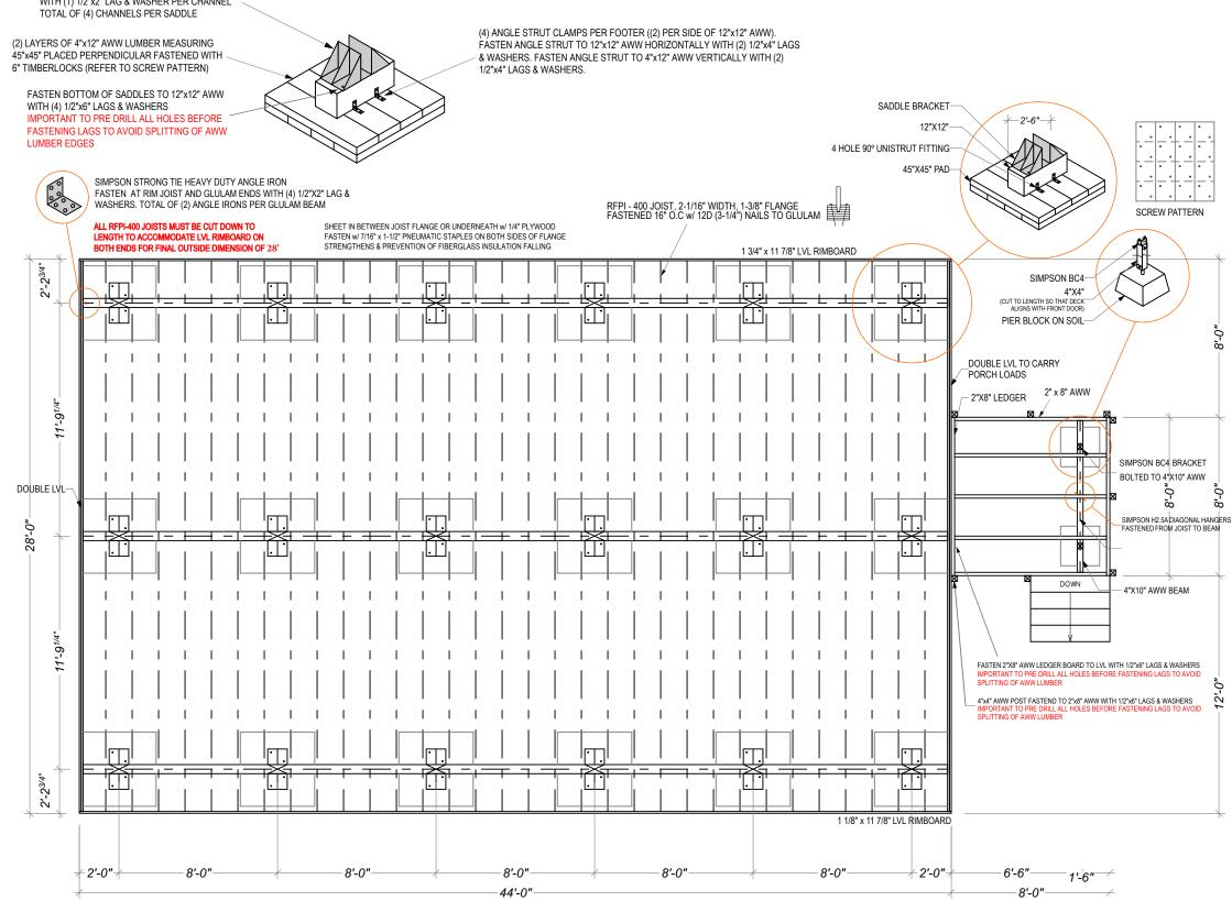
FASTEN SIDE OF SADDLE TO SIDE OF BEAM WITH (1) 1/2"x2" LAG & WASHER PER CHANNEL TOTAL OF (4) CHANNELS PER SADDLE
