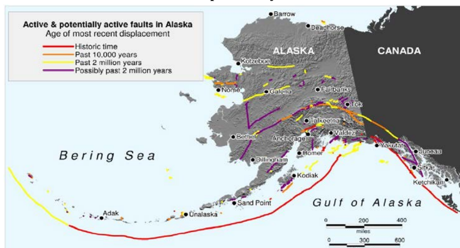
Figure 5-1 Active and Potentially Active Faults in Alaska
