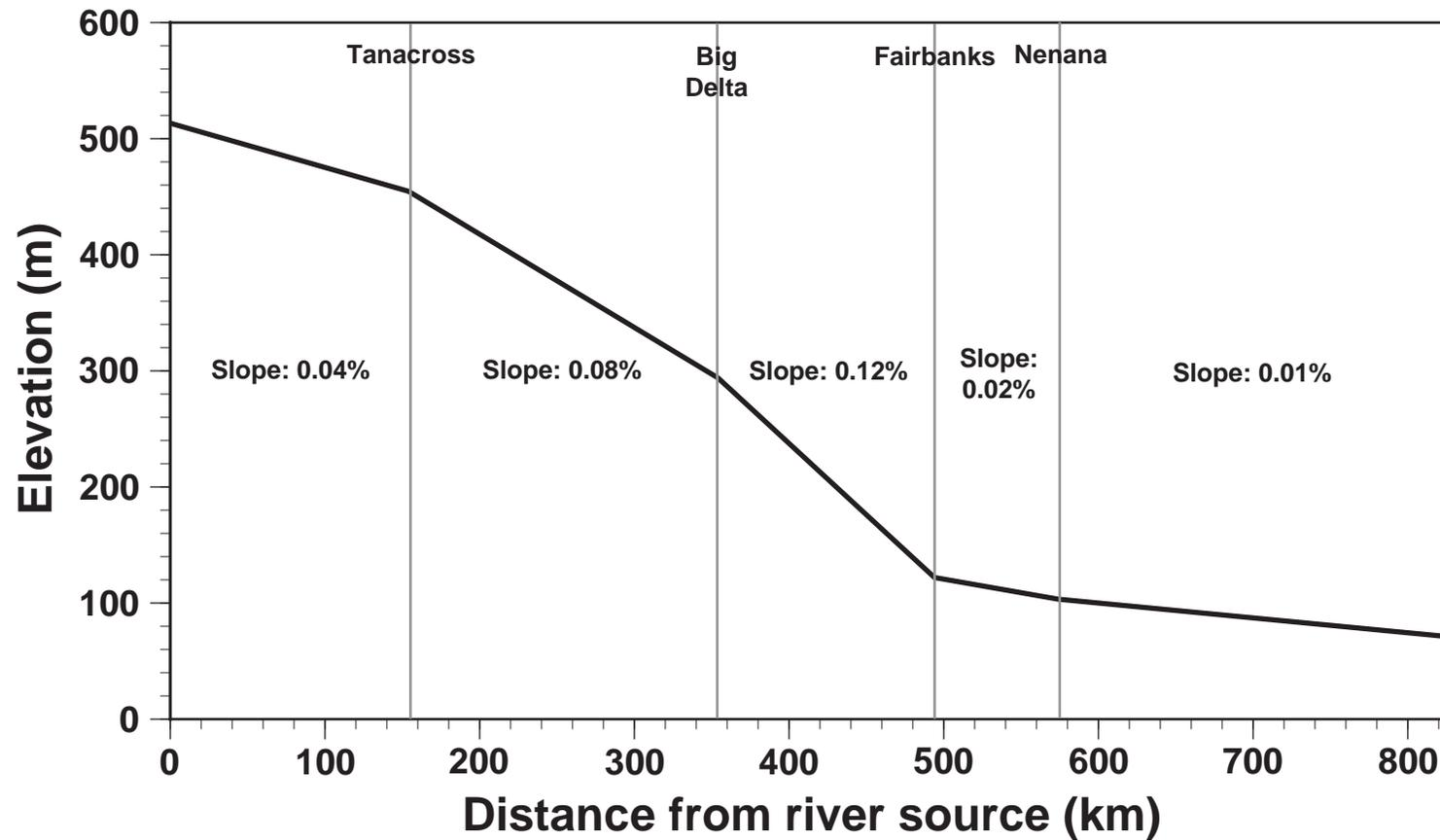
Figure 2. Longitudinal profile of the Tanana River based on published data and elevations of streamflow stations. Approximate locations of settlements with U.S. Geological Survey stream flow stations are shown. Slope values were determined based on the estimated locations of the stream flow stations along the river. (Data sources: U.S. Geological Survey, Anderson 1970)
